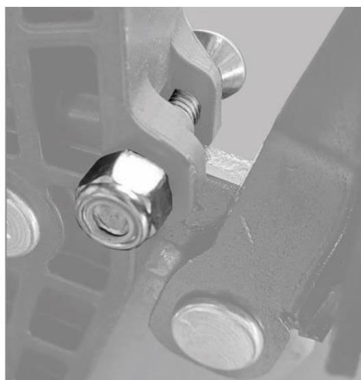
Figure 6 – An Under Torqued Fastener
