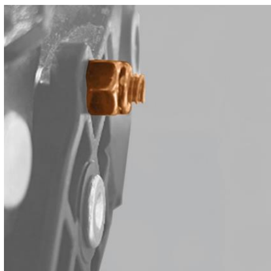
Figure 5 – An Over Torqued Fastener
