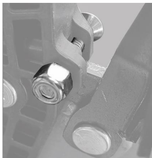
Figure 6 – An Under Torqued Fastener
