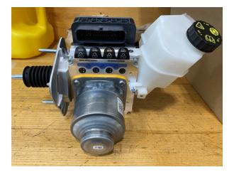
"Dry" IB unfilled: Brake fluid reservoir is empty; brake fluid line ports are sealed with labels.
