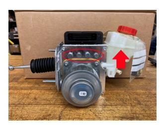
"Wet" IB pre-filled: Brake fluid reservoir is filled (arrow) and brake fluid line ports are plugged with bolts (circled).
