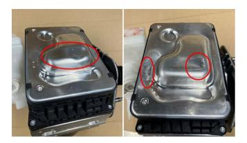
Do not install any part which shows visual damage as shown, or has been dropped from any height.
