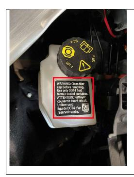
24. For G60 and G70, install the brake fluid label to the reservoir
