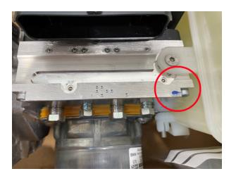
2. Verify the blue mark is located on the new component as shown in the photo.
