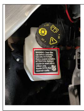
17. For G60 and G70, install the brake fluid label to the reservoir
