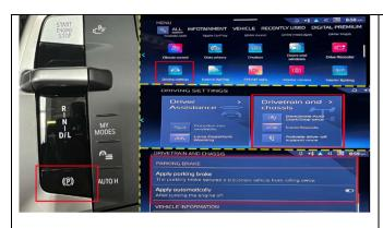
**WARNING:** Prior to releasing the parking brake, secure the vehicle from rolling by raising the tires slightly off the ground using the vehicle lift.
