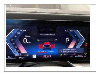
27. Document the odometer mileage in the repair order after the IB has been replaced and successfully programmed and coded to the vehicle.
