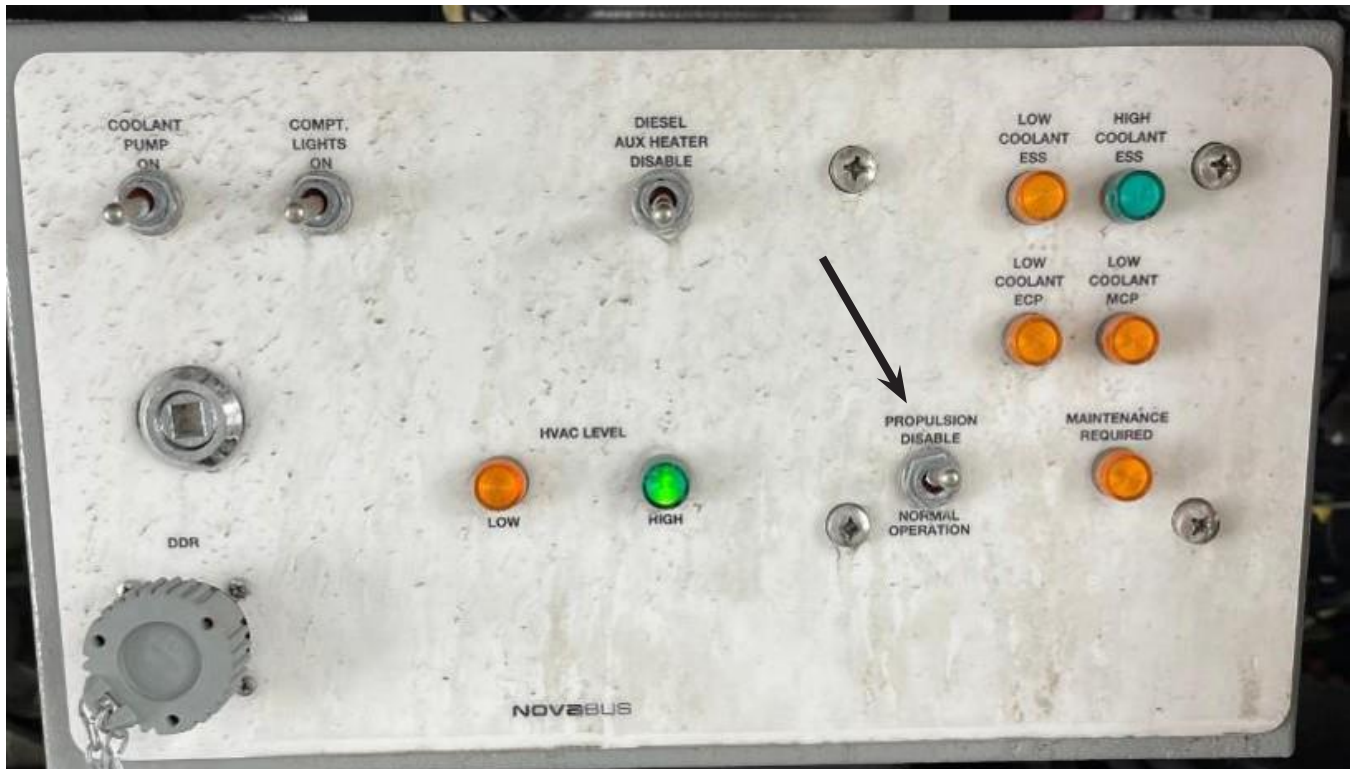
Figure 1 - "Propulsion Disable" Switch, (For Reference Only, Your Configuration May Differ)
