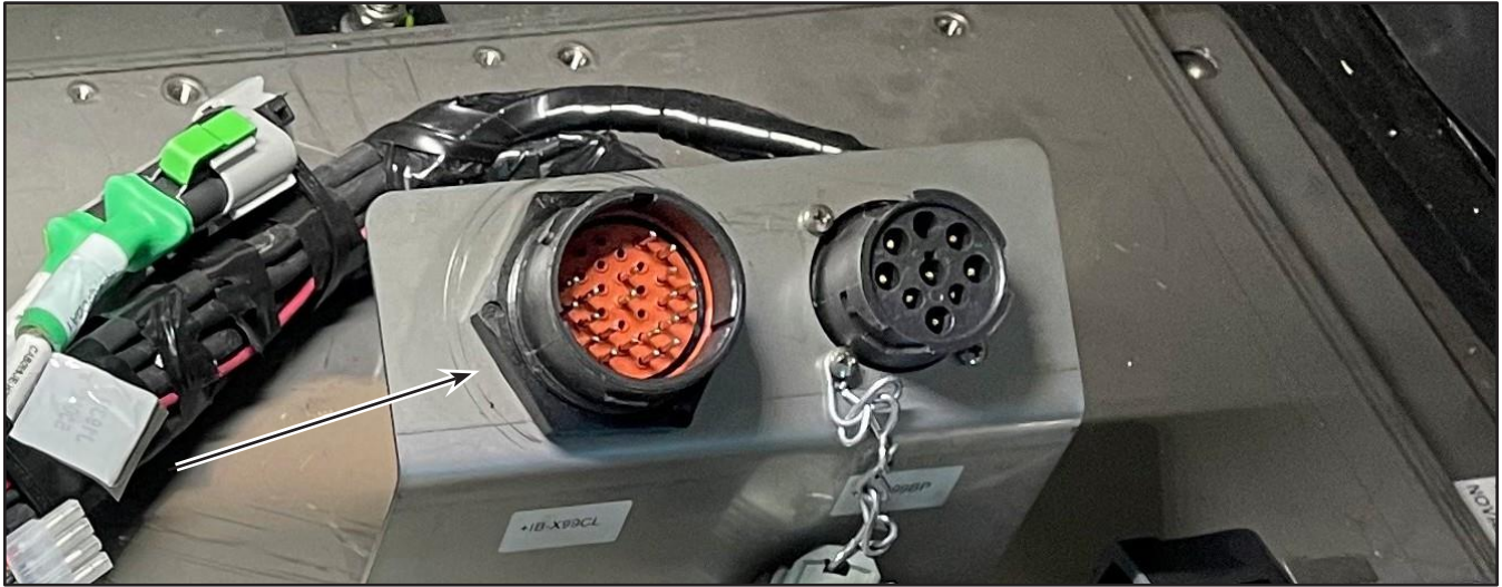
Figure 2 - Locate the Connector (Image for Reference Only, Your Configuration May Differ)
