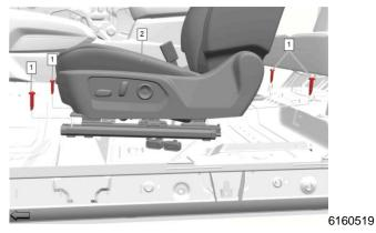
4. Reposition the LH Front Seat. Torque the Front Seat Fasteners to 45 N•m (33 lb ft).
