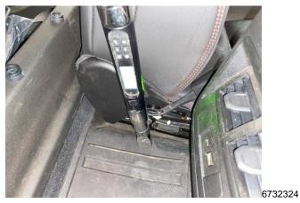
3. Torque the LH Front Seat Belt Buckle Fastener to 45 N•m (33 lb ft).
