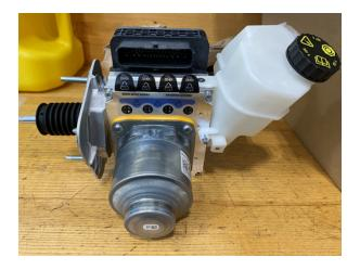
"Dry" IB unfilled: Brake fluid reservoir is empty, and the brake fluid line ports are sealed with labels.
