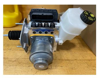
"Dry" IB unfilled: Brake fluid reservoir is empty, and the brake fluid line ports are sealed with labels.
