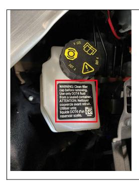
25. For G60 and G70, install the brake fluid label to the reservoir
