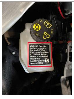
21. For G60 and G70, install the brake fluid label to the reservoir
