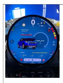
**Note**: The odometer will display 0 miles until the vehicle programming and coding is completed.
