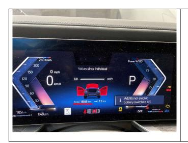
8. Note down the odometer mileage before performing the IB replacement.
