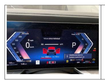
8. Note down the odometer mileage before performing the IB replacement.
