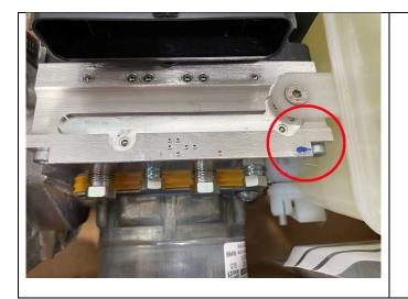
7. Verify the blue mark is located on the new component as shown in the photo.
