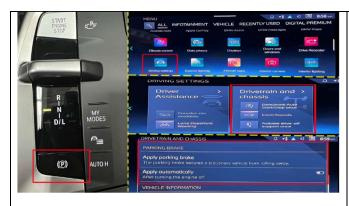
**WARNING:** Prior to releasing the parking brake, secure the vehicle from rolling by raising the tires slightly off the ground using the vehicle lift.
