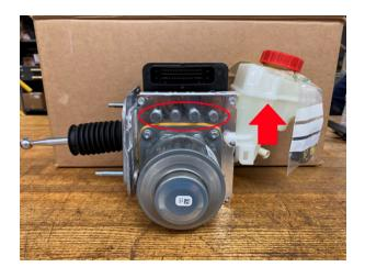
"Wet" IB pre-filled: Brake fluid reservoir is filled (arrow) and the four brake fluid line ports are plugged with bolts (circled).
