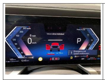
17. The odometer will display 0 miles until the vehicle programming and coding is completed.
