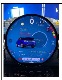
17. The odometer will display 0 miles until the vehicle programming and coding is completed.
