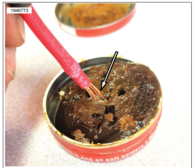
Figure 15. Prep 1: Apply Flux to Stripped Wire
