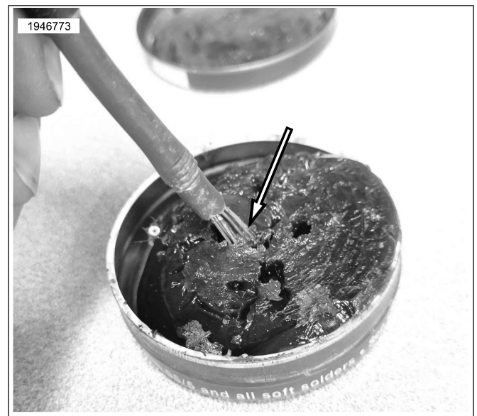
Figure 15. Prep 1: Apply Flux to Stripped Wire
