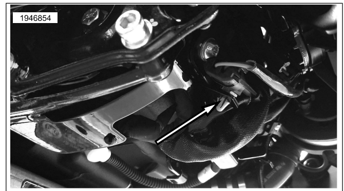
Figure 24. Anchored Cable Strap
