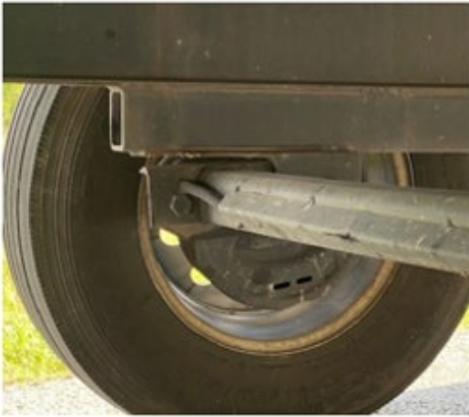
Figure 4 (Axle bracket failure) Follow Repair procedure 2
