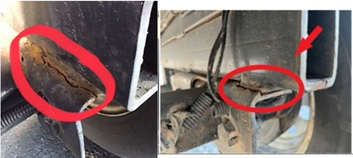
Figure 3 Crack in axle bracket -Follow Repair procedure 2
