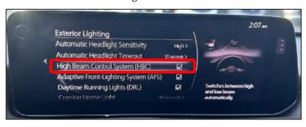
8. Check for presence of High Beam Control Drive vehicle and obtain required photo #2.
