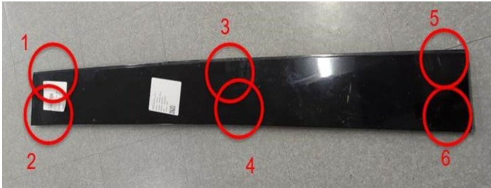
Figure 4 – Front roof applique inspection positions
