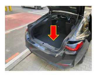
1. Open the tailgate and remove the floor panel (arrow).
