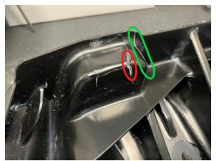
The area in the green circle is OK; it is a normal metal seam/parting line and not to be confused with being a crack.
