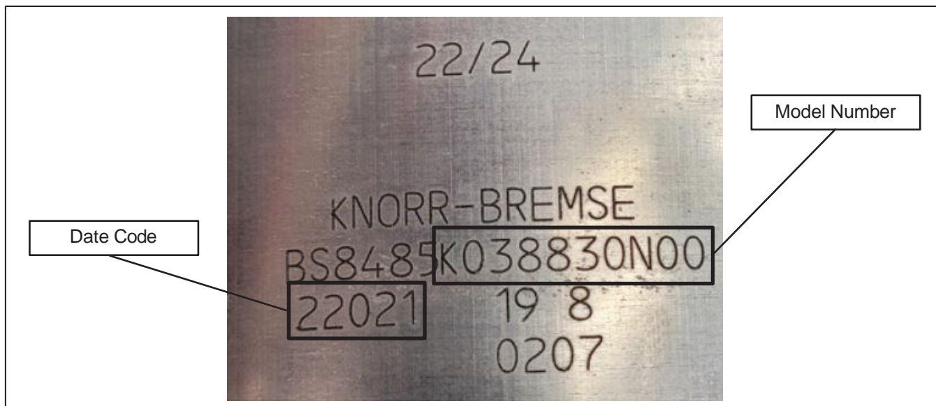
Figure 1 - Stamped Informations on the Brake Chamber
