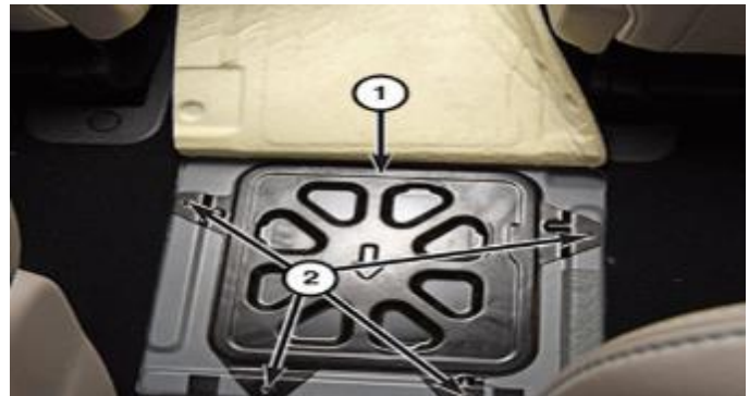
Figure 7 – MSD Access Cover
