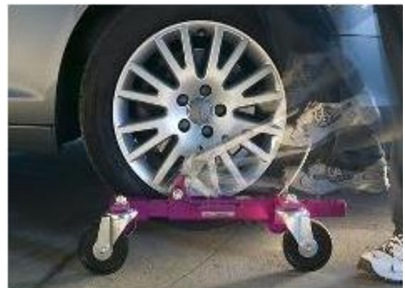
Figure 5 – Wheel Jack Dolly Installed
