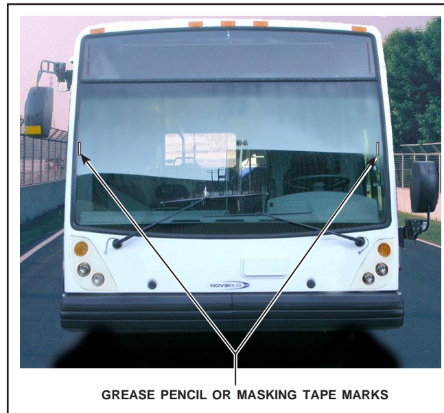
Figure 2 - Windshield Wiper Indicators
