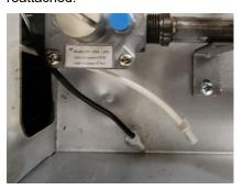
**5.** Locate and unplug the wires from the light switch on the front of the unit, Then remove the light switch by squeezing the locking tabs and replace with the plug provided in the kit (233754).
