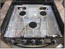
**3.** Locate the red and black wires that connect to the coach wiring (Coach wiring color may vary). Cut this wire directly behind the connector using a pair of electrical cutters.
