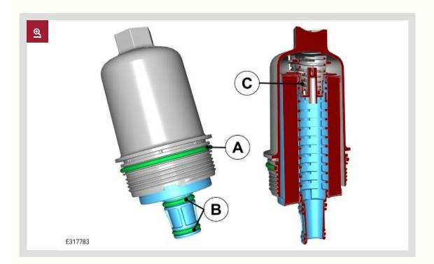
7. Install and tighten the oil filter element cap.
