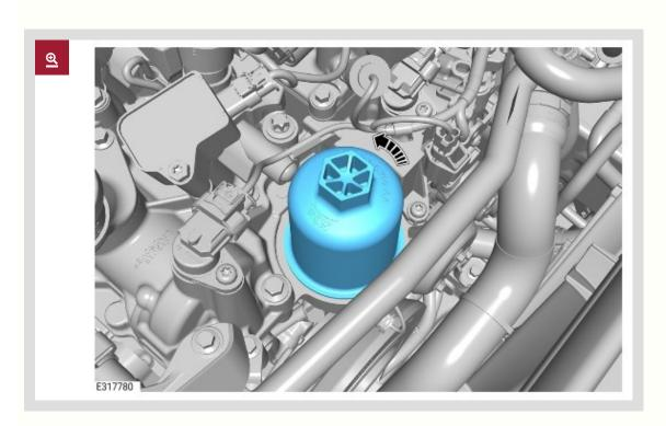
**5.** Remove and discard the oil filter element cap and the oil filter element.
