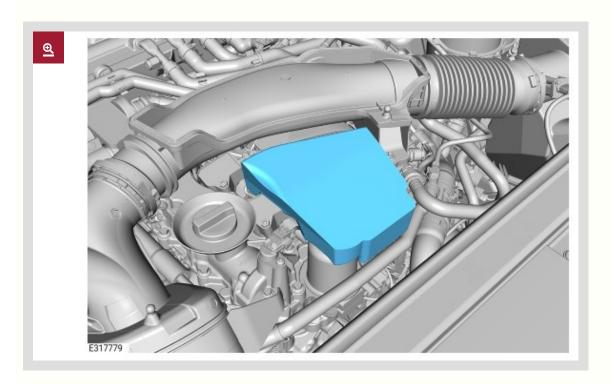
4. Loosen the oil filter element cap 4 complete turns.
