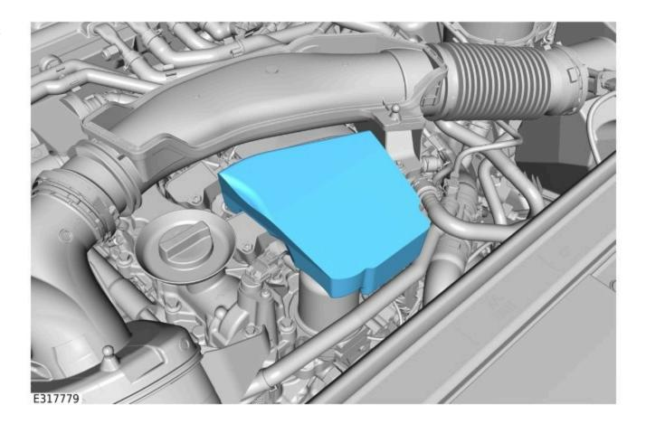
**4.** Loosen the oil filter element cap 4 complete turns.
