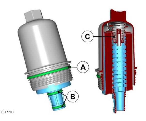
7. Install and tighten the new oil filter element cap.
