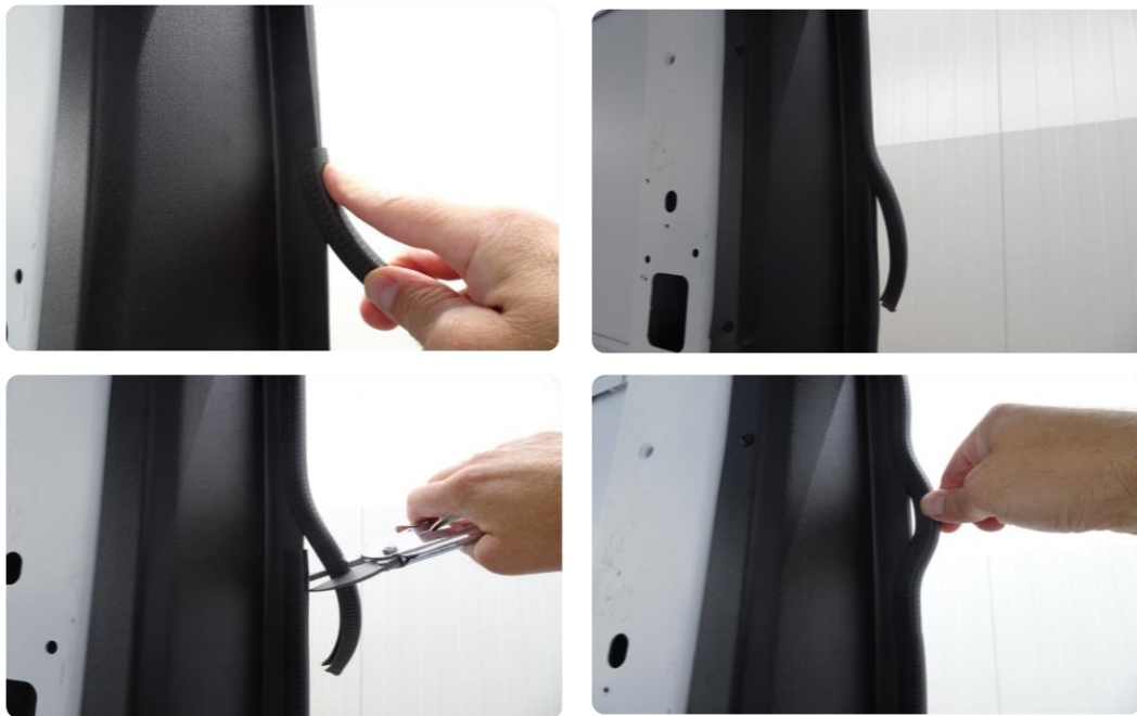
Figure 19 – Window Seal Installation
