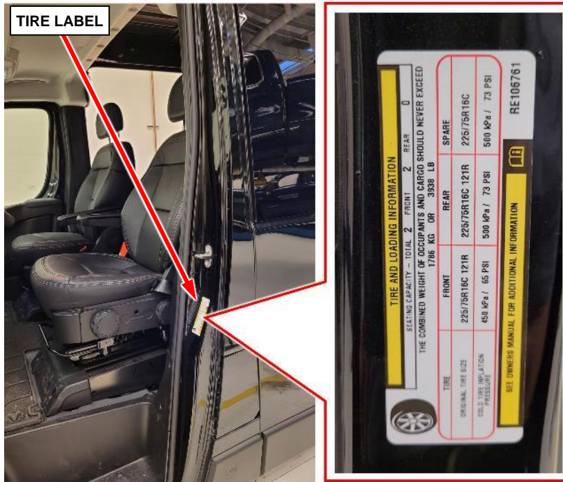
Figure 20 – Locate Tire Label on B-Pillar
