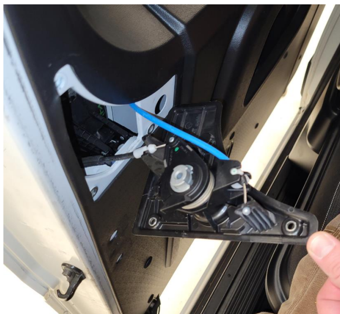
Figure 4 – Door Handle Cables
