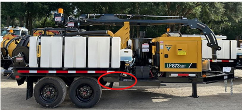
Potential missing stiffener plate location on right side.
