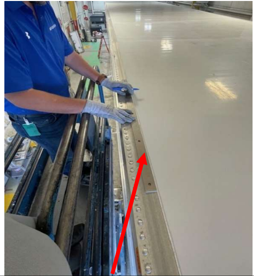
The edge of the Marking Guide should be lined up with the inside edge of the roof Extrusion.
