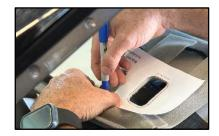
24. Using a glue gun, apply a generous amount of hot glue over the surface outlined area on the headliner.
