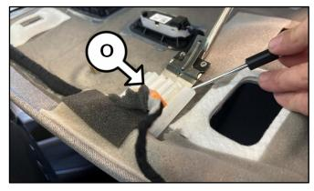
20a. Scrape-off any excess remaining glue from the headliner surface.
