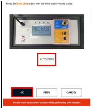
Once 'AUTO ZERO' has completed, the leak test will automatically start.
