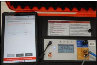
Once the leak test has completed, a 'PASS' result should be displayed on the leak tester
