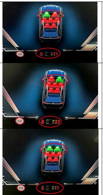
2-Here the image shows the drivers safety belt latch is recognized as latched. This should only occur when drivers' safety belt is connected / latched.
