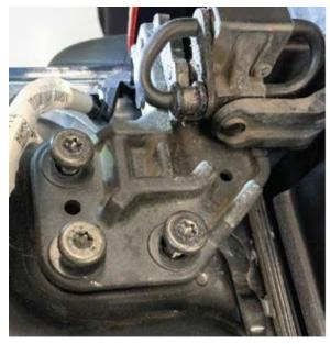
11. With the help of an assistant, lift the tailgate up slightly to allow clearance between the left tailgate lower hinge and the tailgate for the harness to be removed.
