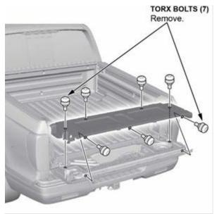
9. Close the tailgate, disconnect the connector, and remove the harness clips.
