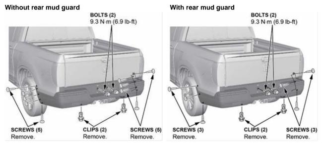
4. Pull out the rear bumper at the wheel arch area to release it from the hooks on the side spacer.
