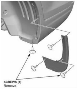
3. Remove the bolts, the screws, and the clips.
