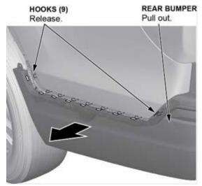
5. With the help of an assistant, release the rear bumper from the hooks on the spacer.
