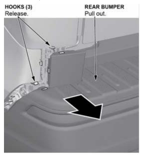
6. With the help of an assistant, pull out the rear bumper to release it from the hooks on the upper brackets. Disconnect the connectors (for some models). Remove the rear bumper.
