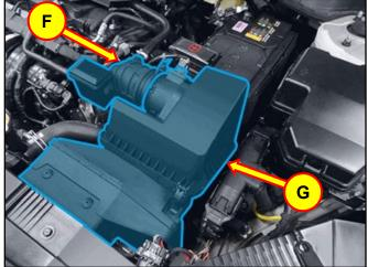
6. Disconnect the air intake hose assembly from the throttle body assembly. (F)
