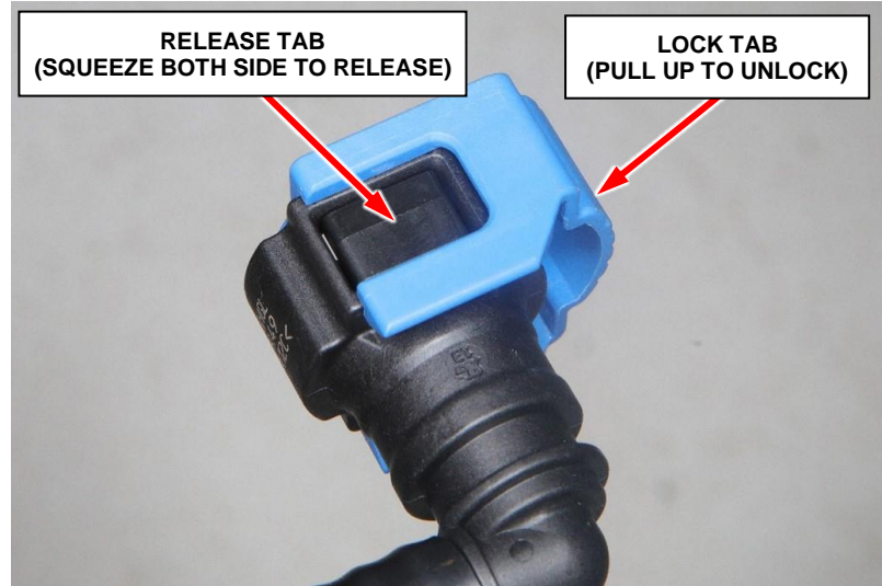
Figure 13 – Upper Fuel Line Lock
