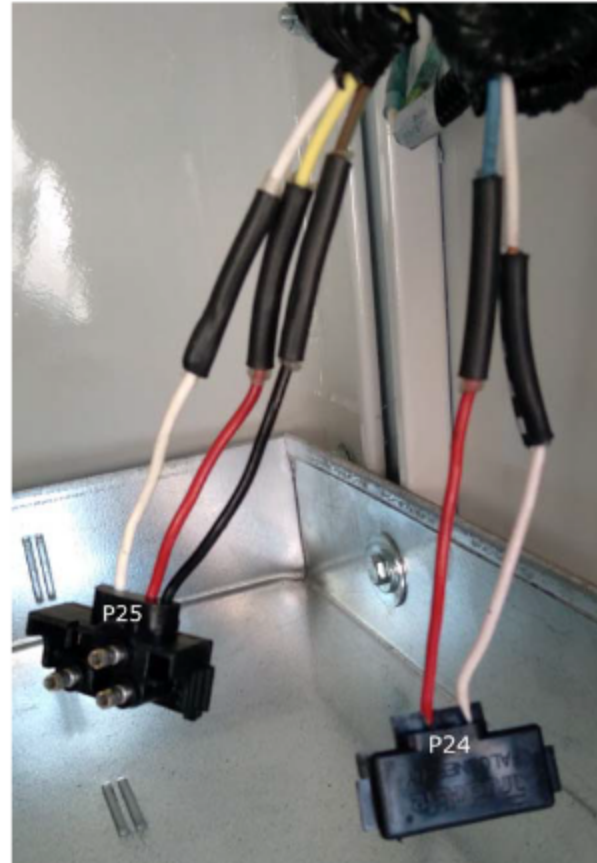
LEFT TAIL LIGHT ORIGINAL WIRING (RIGHT IS SIMILAR)
