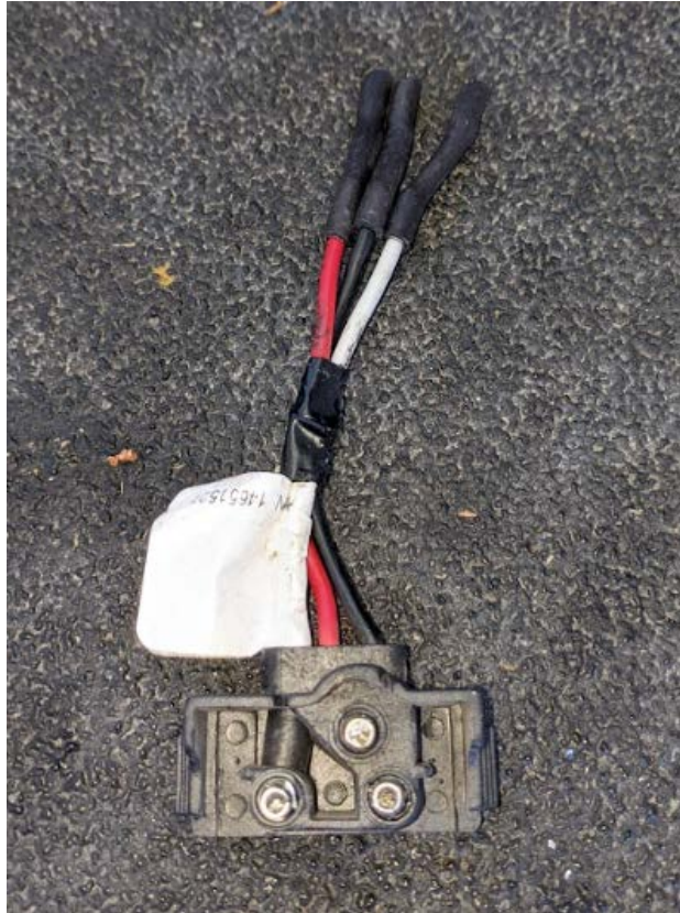
Image 2 – Approx. 4” pigtail remains on connector
