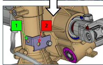
If the harness is secured to the correct (OK) bracket hole (1), then no further action is required. Claim Inspection Labor Op Code 241A17IO.
