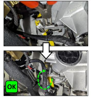
3a. If minor damage to the wire harness insulated wrapping is present (as shown), use a 6" inch strip of Tesa (or 3M vinyl) electrical tape to repair and insulate the open area.
