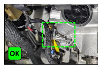
If the harness is secured to the incorrect (NG) bracket hole (2), proceed to the 'Repair Procedure' on page 3.
