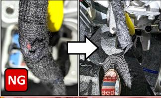
3b. If major damage to the wire harness insulated wrapping/wires is present (as shown), park the vehicle until the replacement wire harness assembly becomes available.
