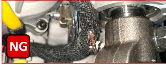
3c. If no damage to the wire harness insulation is present, no further action is required.
