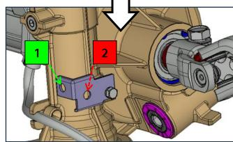
If the harness is secured to the correct (OK) bracket hole (1), then no further action is required.
