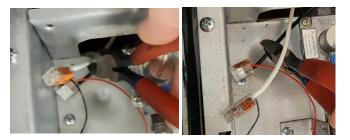
**4.** Crimp the Crimp Caps(233759) to incoming 12V positive and negative to prevent lights from being reattached.
