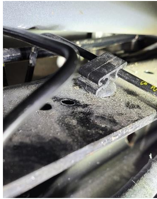
Diagram 4: Retainer clip with rear line uninserted.
