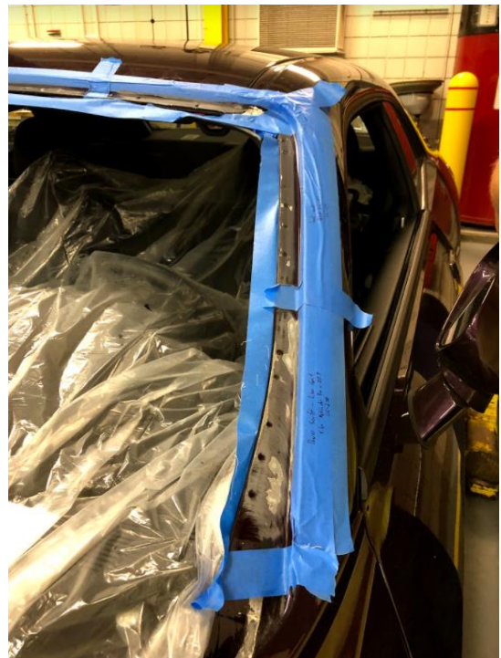
Figure 16 – Protect Adjacent Surfaces
