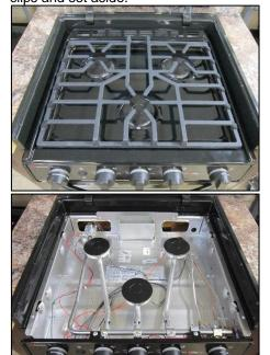
3. Locate the red and black wires that connect to the coach wiring (Coach wiring color may vary). Cut this wire directly behind the connector using a pair of electrical cutters.
