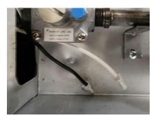
**5.** Locate and unplug the wires from the light switch on the front of the unit, then remove the light switch by squeezing the locking tabs and replace with the plug provided in the kit (0440968).
