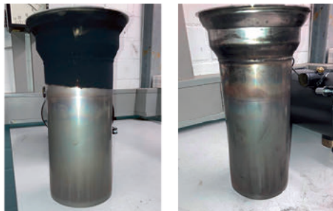
Combustion chamber before ... and after cleaning.
