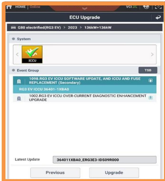
B2. After the ECU Upgrade process shows 100% complete, cycle the ignition key to OFF for at least 10 seconds to reset the control unit.
