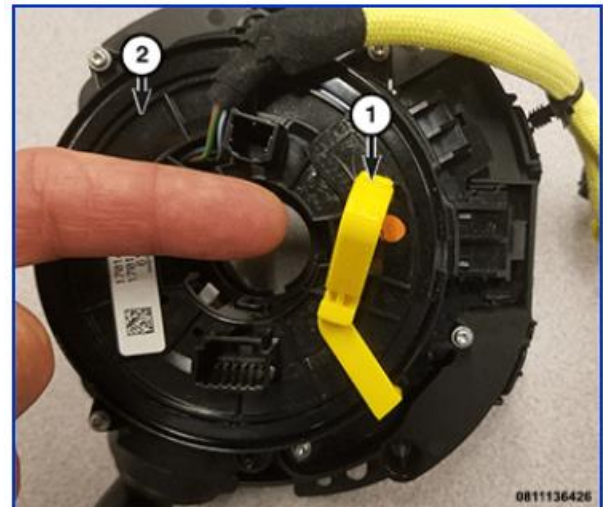
1 - Lock 2 - Clockspring Rotor
