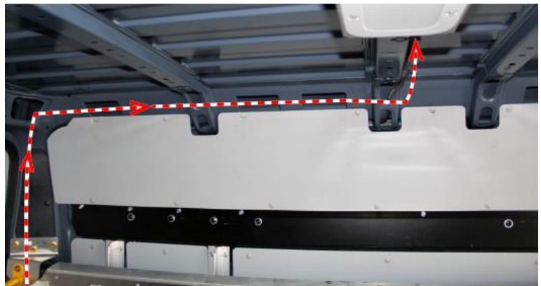
Figure 6 – Dome Light Power Wires Routed Up D-pillar to Dome Light
