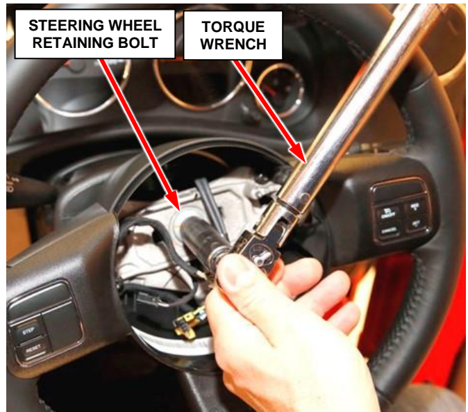
Figure 13 – Tighten Steering Wheel Retaining Bolt to 40 ft. lbs. (54 N·m)
