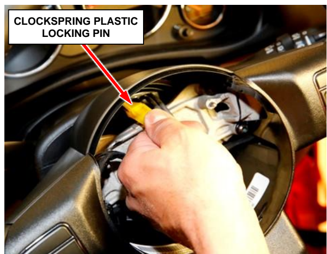
Figure 12 – Remove Clockspring Locking Pin
