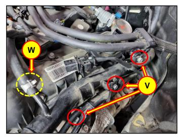
23. Remove the brake vacuum hose mounting bolt (X) and water inlet side mounting bolt (Y), and then remove the water outlet pipe.
