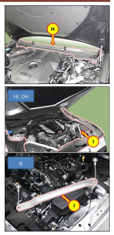
10. Remove the front strut bar (I).
