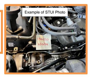
37. Reinstall the LH turbocharger water pipe and hose.
