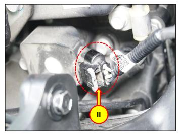
31. Release the wiring protector locks (JJ) and lift the protector.
