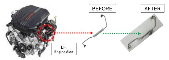
Follow the procedure outlined in this bulletin to replace the oil feed hose and pipe assembly with an updated oil feed pipe assembly (full stainless steel type).
