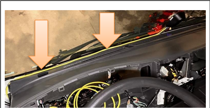
Figure 16 Camera cable to be removed from behind the instrument panel (shown in Yellow).
