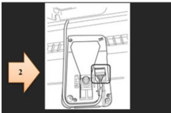
**Note: Pay attention to the camera/cable connection and note the position in which the cable is connected.**
