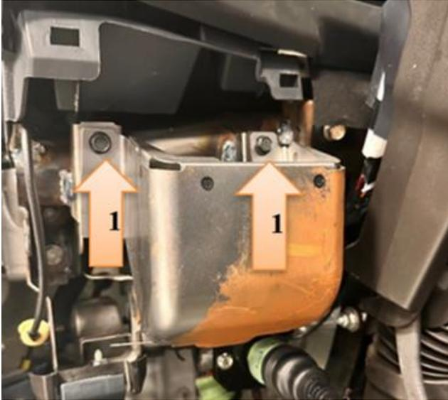
47. Remove the two (2) 10mm bolts and remove the knee bracket.
