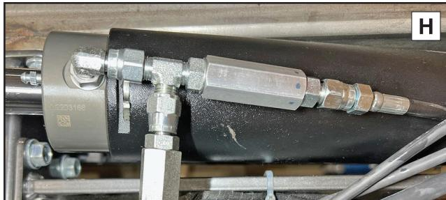
10. Connect flow restrictor to tee connector and connect hydraulic hose to flow restrictor. Tighten to snug. See Photo H.
