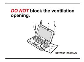
b) **DO NOT** block the ventilation opening for the cooling fan of the personal computer.
