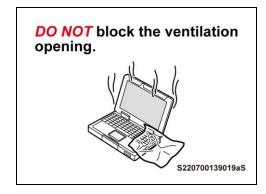
c) **DO NOT** block the ventilation opening for the cooling fan of the personal computer.
