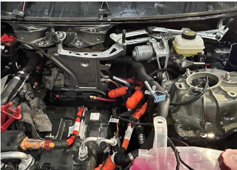
Figure 7, HV electrical connectors with protective covers (001 589 06 91 00)
